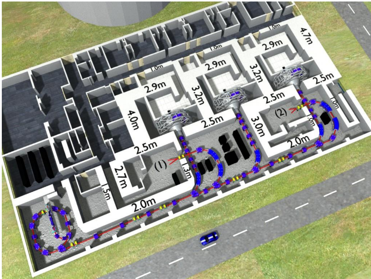
2553 Figure 3.18. Proton therapy facility at the Loma Linda University Medical Center. The installation has a 2554 synchrotron, three rooms for treatments with a gantry, and a fixed beam branch with two beam lines (1) 2555 and a fixed beam line for calibration measurements (2) (Courtesy of G. Fehrenbacher, J. Goetze, T. 2556 Knoll, GSI (2009)).
