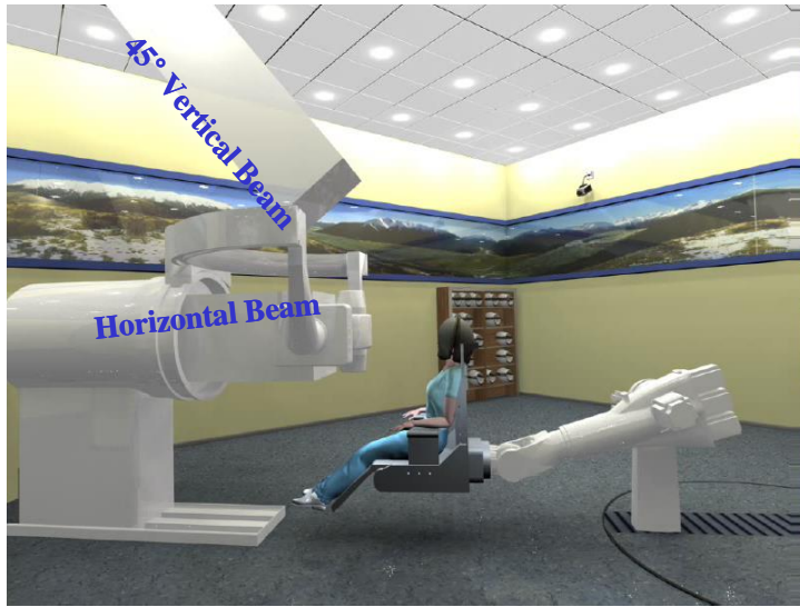
1450 Figure 2.13. Fixed beam room with dual beams (Courtesy of Siemens Medical Systems)
