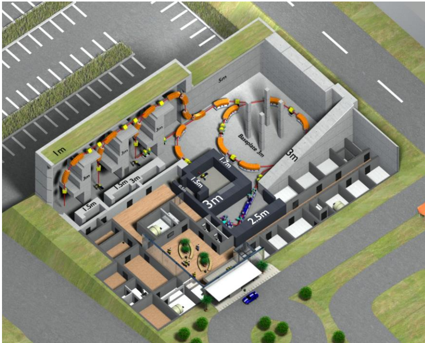
2732 Figure 3.25. Layout of the Gunma ion irradiation facility with the LINAC, the synchrotron (ring 2733 accelerator), and the treatment rooms (Courtesy of G. Fehrenbacher, J. Goetze, T. Knoll, GSI (2009)).
