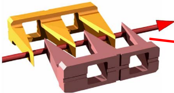
Multiple wedge degrader 238-70 MeV (PSI) 5 mm \Delta Range in 50 ms
