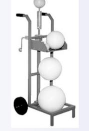
LUDLUM neutron ball cart model 42-5 (diameter: bare, 2", 3", 5", 8", 12")
