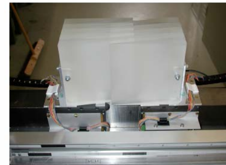
Fig. 1: Prototype of PMMA-wedge system for fast, passive energy modulation compensating the longitudinal component of target motion.
