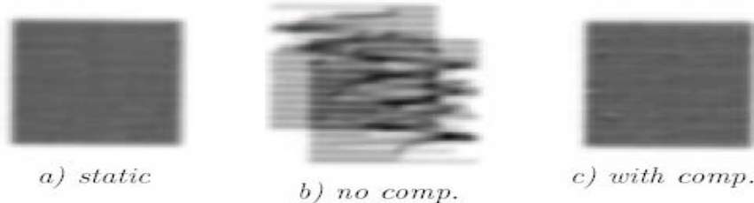
Fig. 2: Test of lateral compensation accuracy. A homogeneous pattern (a) is irradiated while an x-ray sensitive film is moved in a respiration-like 2D pattern. The strong motion effect (b) could automatically be compensated (c) by the prototype setup.
